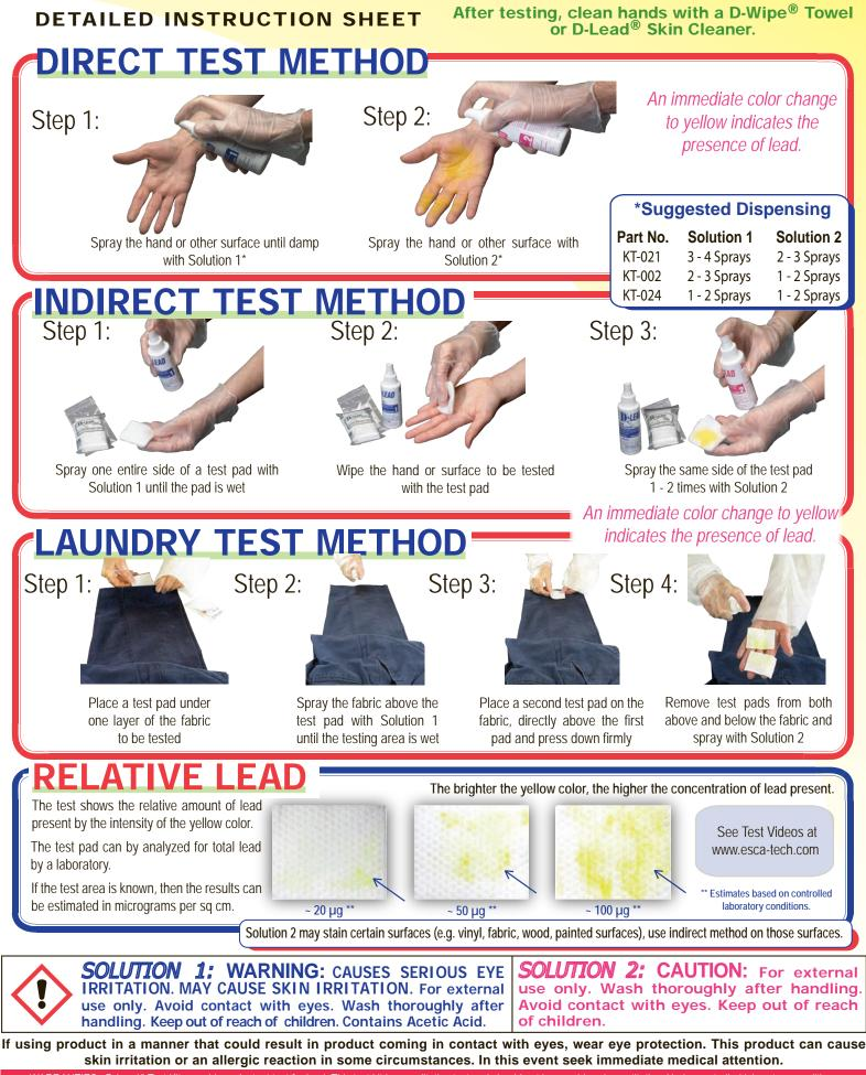
WARRANTIES: D-Lead® Test Kits provide an instant test for lead. This test kit is a qualitative test and should not be considered quantitative. Under controlled laboratory conditions D-Lead® Test Kits have consistently detected 20 micrograms total lead. Under conditions described in the directions D-Lead® Test Kits will detect high levels of leachable lead. The use of this kit is not intended to replace a professional inspection. No guarantees are intended or implied.
